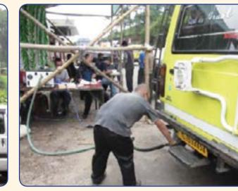
**Emission test of Diesel driven vehicle in progress**
